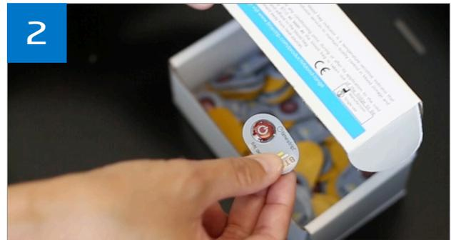
BT10 does not require pre-conditioning and can be activated at room temperature: keep box in a drawer before use and it can be easily taken out at the time of use.
